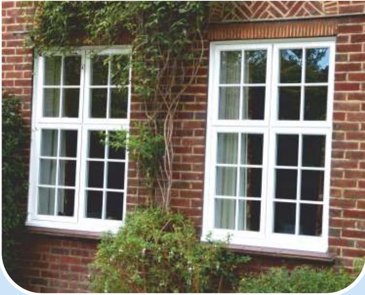
With their authentic 45° angled putty-line design our Putty-Line windows are the perfect solution for replacing old putty glazed steel windows. The window has been specially designed to replicate the appearance of traditional putty glazed windows, whilst offering superior security, weather and thermal performances. They use a 'Polyamide' thermal break and double glazed Argon filled sealed units to achieve excellent thermal values.
