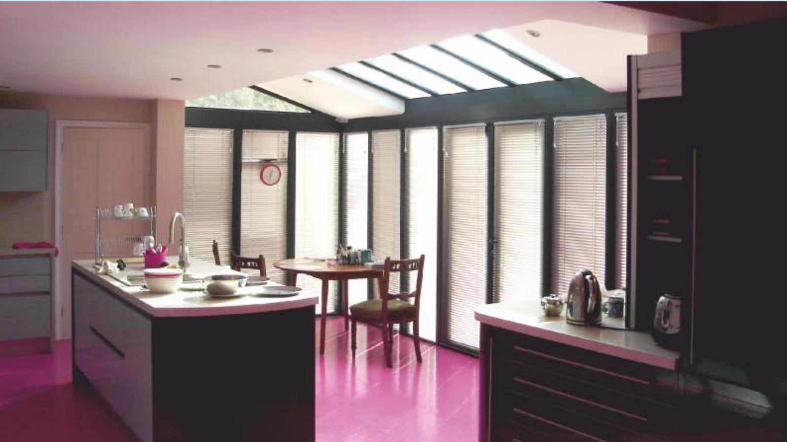
The superior natural strength of aluminium allows for a much larger glazed area with the structural integrity and strength to take several inches of snow and wind speeds of more than 100mph. This roof system is an energy efficient thermally broken system that is suitable for both commercial and domestic purposes.
