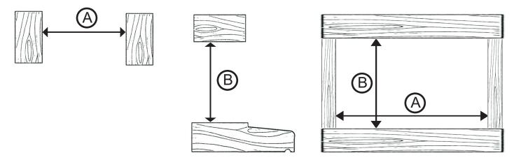
The above shows a typical timber type subframe aluminium window application. To obtain long leg aluminium manufacturing / ordering sizes, the measures A and B are tight inside timber sizes, then please use dimension C from the table.
