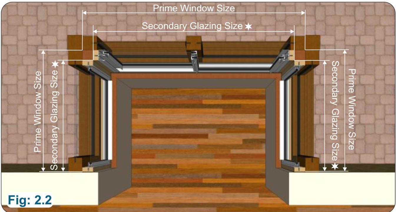
Fig 2.0 Shows a cut through of a square bay window with secondary installed.
