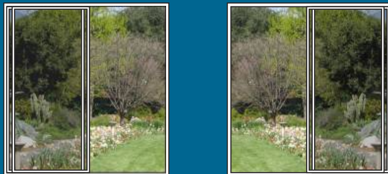
← BOTH PANELS CAN SLIDE → TO THE LEFT OR RIGHT APPROX 50% CLEAR OPENING
