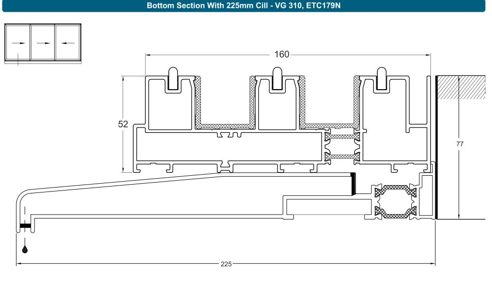
Showing Internal Floor Levels And Drop Required To Create Flush Floor Levels
